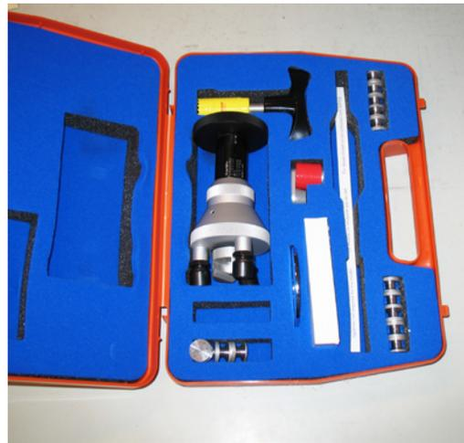
Elcometer Paint Adhesion Tester
