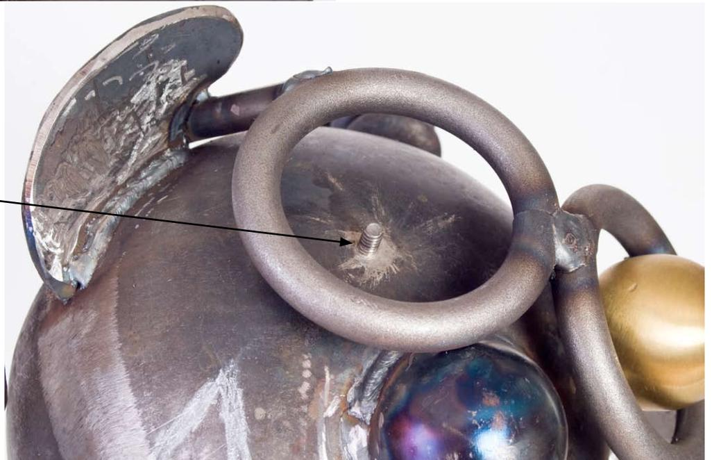
The ¼” steel plate and the 2” fence termination-weld on (Item No. 46-3221-C) was attached using brazing rod. For painting purposes I was wanting a more defined line between the two items. Brazing provides a more well defined line when compared to welding.
